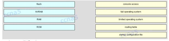
console access -> Not Scored full operating system -> flash limited operating system -> ROM routing table -> RAM startup configuration file -> NVRAM
